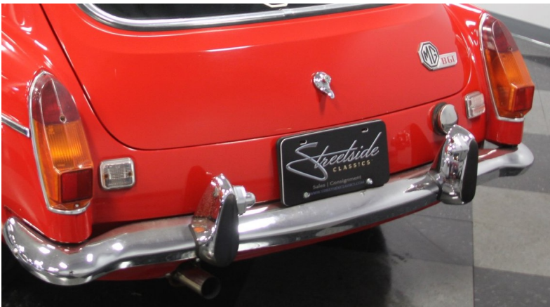
MGB Tail 1973 Chrom Bumper with Rubber MG Badge black/blue, /black, /red Nummernschildbeleuchtung an den Bumpnern
