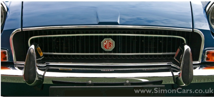
MGB Front 1970 - 1972 Recessed Grill (Haifischmaul) MG Badge octal red Chrom Bumper with Rubber
